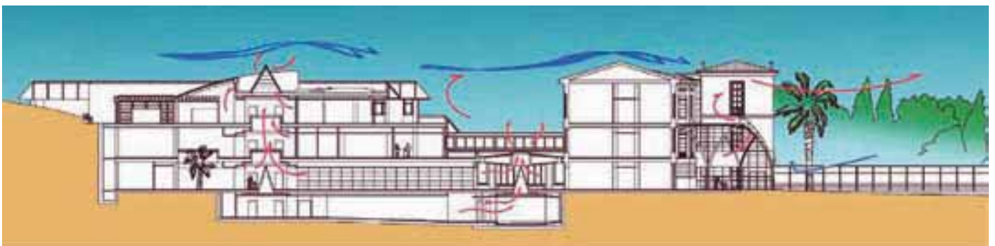
Visualisation of wind driven and thermal buoyancy effects at Meyer Children's Hospital (Italy)
