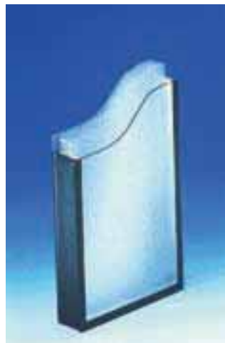
Transparent insulation from Okalux, (49 mm). U = 0,8 \text{ W/m}^2\text{K} , g_{dir} = 80\% , g_{dif} = 60\%
